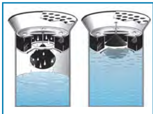
Floor drain float plug.
