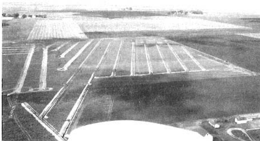
Figure 5. Aerial view of lateral tile system in LRA 103.
