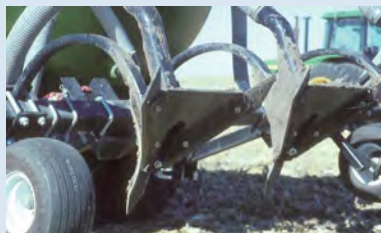
Closeup of injectors.
